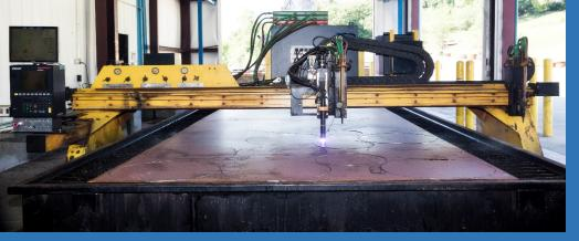
First, PRESCOR starts with burning precise circles with state of the art CNC machines.
