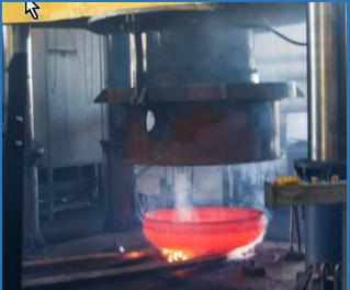
Once the disk is at the appropriate temperature it moves immediately to a press and hot formed seamlessly.
