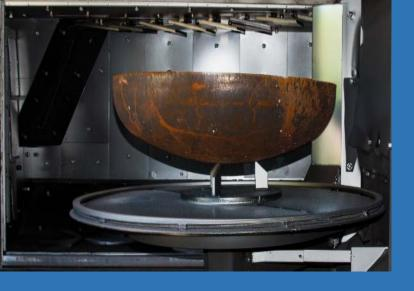
Then, the newly formed head is moved to the blaster. All of PRESCOR's heads are descaled (shot blast for carbon and low-chrome alloys and sand blast for stainless steels, high nickel alloys, and some "exotic" plates).
