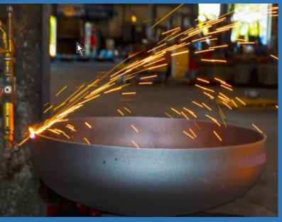
Lastly, all heads are beveled to our customer's specifications. Every tank head PRESCOR manufactures has the strength and consistency to perform flawlessly when fitted to your pipe or shell.
